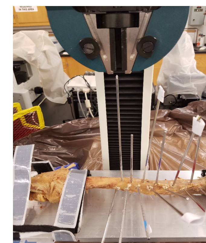
Figure 4: Demonstration of testing pull out strength of the pins
