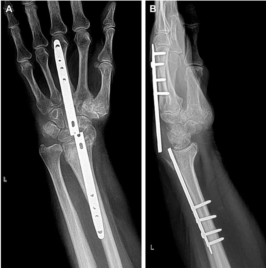
Fig. 11. Fatigue failure of the plate through the middle screw holes of the plate on the (A) anteroposterior and (B) lateral radiographs.
